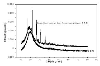
Figure.1.XRD patterns of SBR and chemically modified SBR
