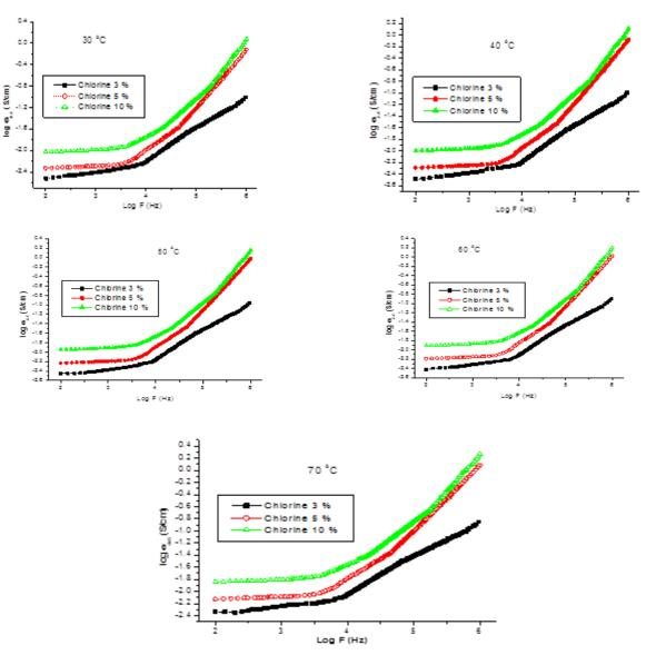
Figure.4.AC conductivity of MSBR with different content of Cl @ various temperatures
