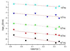
Figure.5.Variation of log  $\sigma_{AC}$  with 1000/T (K<sup>-1</sup>) of 3% Cl sample
