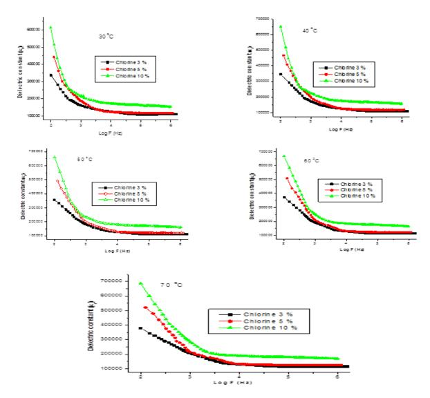
Figure.8.Dielectric constant of modified SBR at different temperatures
