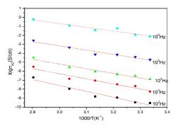
Figure.6.Variation of log  $\sigma_{AC}$  ( $\sigma_{AC \text{ in } S/cm}$ ) with 1000/T (K<sup>-1</sup>) of 5 % Cl sample
